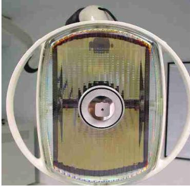
Before glueing the miniature camera stand to your dental light all the adhesive surfaces of the light and stand baseplate must be cleaned and degreased with alcohol and a clean cloth.
