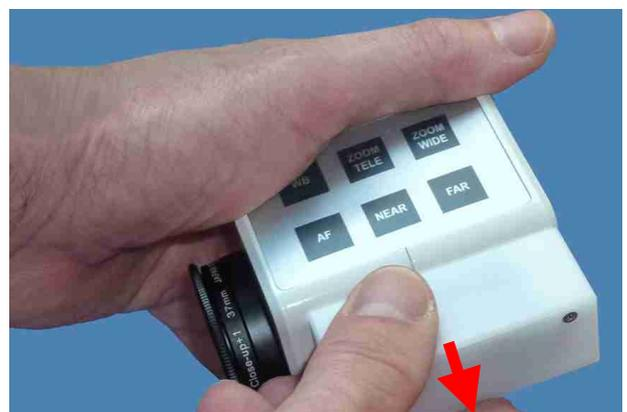
To unplug the receiver box pull the box straight off the connector without turning the box against the camera body.
