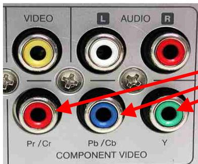
Connect the three RCA plugs of the camera cable to the component (green, red and blue) RCA input sockets of your HD monitor. As the input source of your monitor choose "component". Most modern HD TV devices have component inputs.
