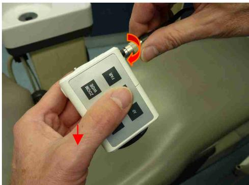
Please, at first connect the 6pin camera cable plug with the socket on the camera housing. Since this is possible in one position only, you should turn the camera in your left hand against the cable plug in your right hand in opposite directions, until the plug engages.
