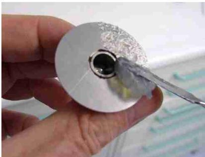
With a cement spatula a thin layer of Hylosil<sup>®</sup> silicone glue is spread onto the surface of the stand baseplate. For dental lights with a relief on their front side (e.g. Siemens M1, Sirona E, Pelton Crane etc.) the silicone layer must be somewhat thicker. The stand fed with silicone adhesive is put on the center of the light front and pressed on slightly, until some silicone outpours the baseplate at the edges.
