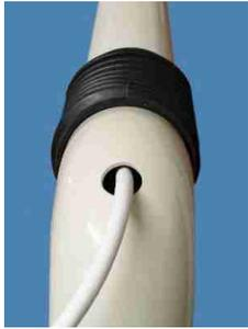
**Please notice:** For laying the camera cable inside the inner tube of the dental light one has to drill a small hole into the front side of the dental light tube (often plastic parts). This bore hole will lead your dental light to lose its registration and warranty (medical products law). We leave it up to you to drill this hole by yourself or have a technician from your dental supplier drill this hole and lay the cable for you.
