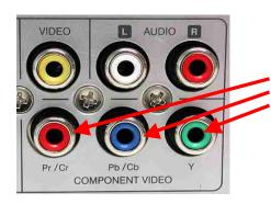
Connect the three RCA plugs of the camera cable to the component (green, red and blue) RCA input sockets of your HD monitor. As the input source of your monitor choose "component Most modern HD TV devices have component inputs.
